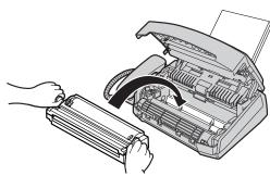
Close the front cover, until locked, by pushing down on both sides.
